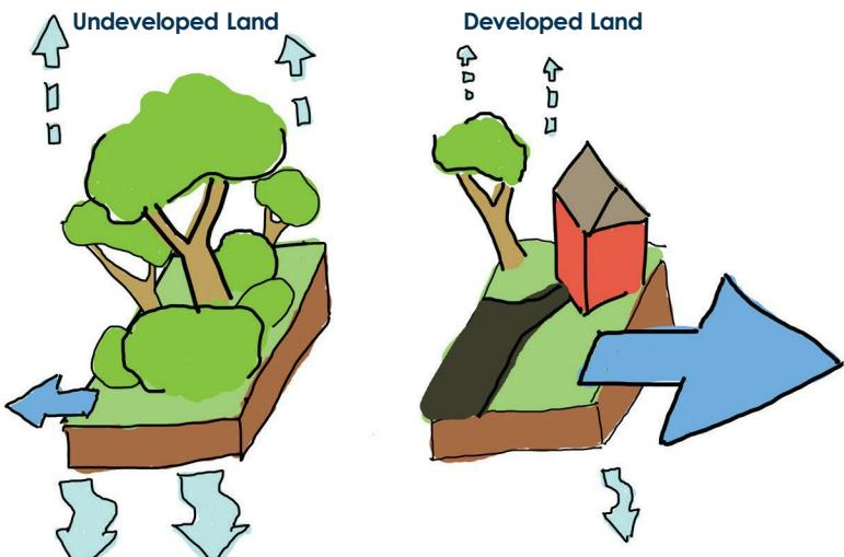
When it rains on an undeveloped piece of property, much of the rainwater infiltrates into the soil or is evapotranspired back into the atmosphere. When vegetation is replaced with streets, driveways, sidewalks, houses, and lawns, less rainwater is able to infiltrate or return to the atmosphere, and more of the rain turns into runoff.
