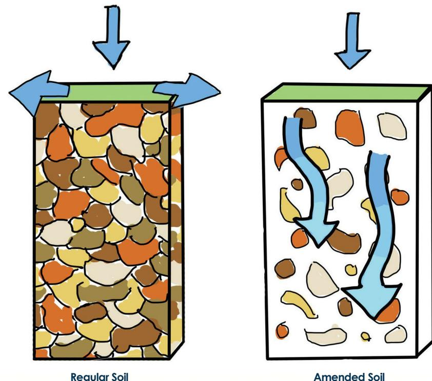
There needs to be air spaces in between soil particles for water to be infiltrated. Amended soils have increased air space, but these air spaces are lost if the soil is compacted by heavy equipment or vehicle parking.
